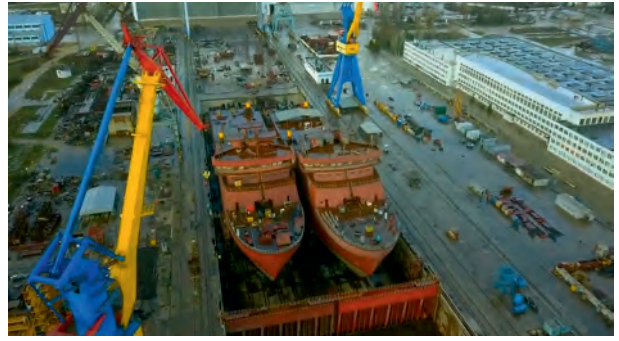
The dry dock of the Zaliv shipyard. The construction of the two cable vessels of Project 15310, Volga and Vyatka, for the Black Sea Fleet of the RF. The deadweight – 8,000 tons, the length – 140 metres, the width – 19 metres, the completion is rescheduled for 2021-2022. The photo from the BlackSeaNews archive, January 2020
